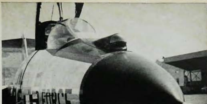
Interceptor IR installation
