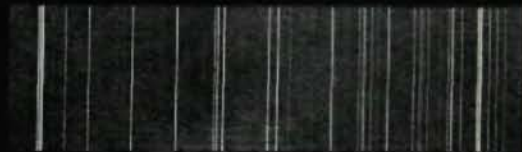
A typical 2nd order spectrum of 1 sec. exp. with 10 micron slit indicates:
