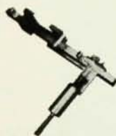
Atomic Beam Spin Analyzer (for Stern-Gerlach Experiment)
