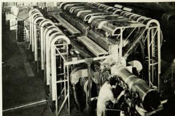
Fig. 2. Overhead view of the Astron induction accelerator (4 MeV, 150-ampere electron beam).
