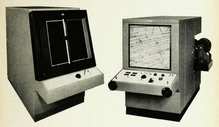
ITEK CUSTOM IMAGE PLANE DIGITIZER . . . specifically designed for digitizing spark chamber photographs or filmed phenomena . . . measurements in X and Y are made directly from the image plane of the projected film.
