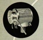
DETECTOR. Vacuum mounted • high sensitivity photomultiplier tube mounted external to vacuum • detects radiation through a wavelength range from 500A to 6,000A.
