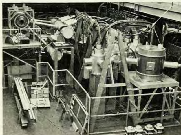
Fig. 9. A photograph of the equipment which has been assembled for magnetic pumping. The ceramic section through which the plasma would pass is seen on the platform at the left.
