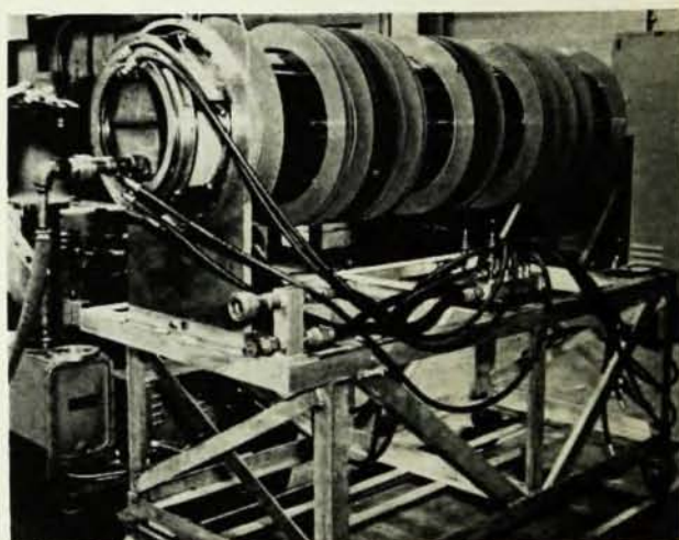
Fig. 11. Plasma lens at BNL. Longitudinal stabilizing windings shown
