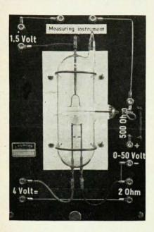
This new laboratory experiment permits the student to observe the transitions which result from the inelastic collisions of electrons with mercury and neon atoms. These various transitions are observed by both spectroscopic and electrical methods.
