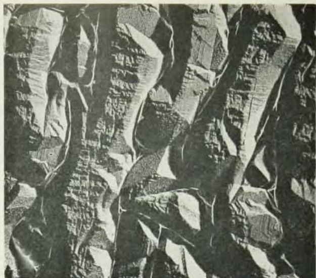
Gallium-arsenide film sputtered on germanium substrate
