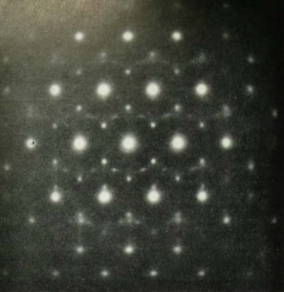
Electron diffraction pattern of Au-Ni alloy film grown epitaxially on (100) NaCl inclined several degrees to [001]-zone axis. Extra spots were caused by twin lattices and double diffraction.
