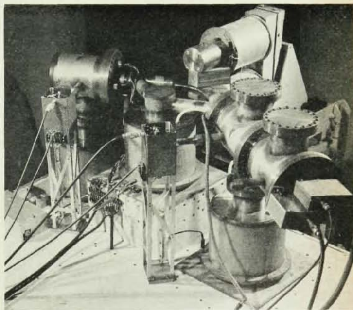
Fig. 2. All-metal ultrahigh-vacuum system for studies of electron ejection from surface by ions. Mercury diffusion pumps with LN traps.
