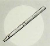
Tempilstik° The most widely used Tempil°product for determining temperatures . . . Marks like a crayon on workpiece—melts when specified temperature is reached. Response delay: of the order of a millisecond.
