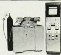
6 .5 METER SCANNING MONOCHROMATOR SEYA-NAMIOKA RANGE 300A - 6,000A*
