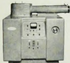
14 1 METER SCANNING MONOCHROMATOR SEYA-NAMIOKA RANGE 300A - 6,000A*
