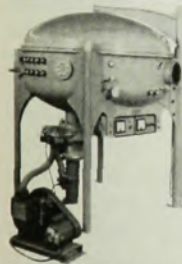
13 1 METER SPECTROGRAPH FIXED POSITION RANGE 500A - 4,000A*
