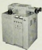
9 1 METER SCANNING MONOCHROMATOR SEYA AND NORMAL INCIDENCE RANGE 300A - 6,000A*
