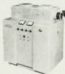
11 1 METER NORMAL INCIDENCE SCANNING MONOCHROMATOR MCPHERSON TYPE RANGE 300A - 6,000A*
