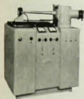
8 2 METER GRAZING INCIDENCE VACUUM U. V. SCANNING MONOCHROMATOR, ROWLAND CIRCLE RANGE 50A - 2,000A*
