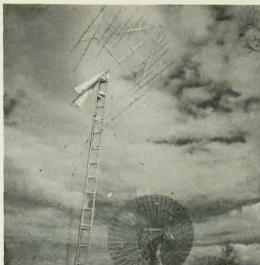
Log periodic antenna (for studying refraction and scintillation of radio stars) and 84-foot and 28-foot parabolas of Air Force Cambridge Research Laboratories, Sagamore Hill Radio Observatory, Mass.
