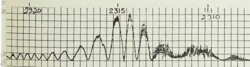
Passage of Transit IV A (54 Mc) into auroral regions on October 4, 1961. Nulls are Faraday rotations; heavy black fluctuations are scintillations. Both geographic and geomagnetic latitudes are given.
