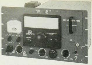
PG-650-C versatility has again been extended to include operation as a modulator or amplifier for pulse and C. W. operation. All the original features of high power, high frequency range and stability have been retained to give this unit its outstanding position as a basic requirement in research work in ultrasonics and nuclear magnetic resonance.
