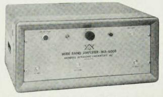
This amplifier allows coverage from 6-60 MC while performance under any conditions of pulsed operation is exceptional due to the quick recovery time. An R.F. output and pickoff point allow direct presentation of the signals and mixing with other systems.
