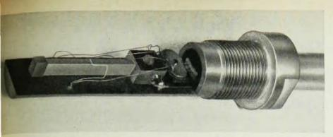
elegant, but tiny refrigerator, utilizing Nernst-Ettingshausen effect, has been monstrated in the Solid State Physics boratories at Lockheed Missiles & Space mpany. This type of cooling is appliable below 200° Kelvin, where thermoctric cooling is no longer efficient. It the particular promise for space appliation because of the reliability inherent its all-solid state construction.
