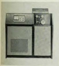
CV SERIES CHAMBERS AND PS SERIES PUMPING SYSTEMS The results were our CV-18 and CV-14 vacuum chambers and our PS-62 and PS-42 pumping systems. (Same basic units—the chambers have baseplate and bell jar. CV-18 and PS-62 units use 6-inch diffusion pumps; smaller CV-14 and PS-42 units use 4-inch pumps).
