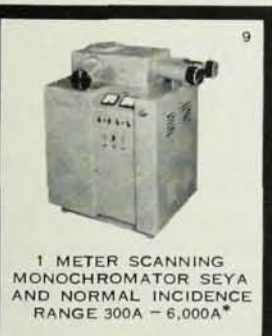
1 METER NORMAL INCIDENCE SCANNING MONOCHROMATOR ROWLAND CIRCLE, RANGE 300A - 6,000A*
