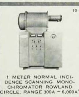
1 METER NORMAL INCIDENCE SCANNING MONOCHROMATOR MCPHERSON TYPE RANGE 300A - 6,000A*
