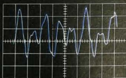
LEFT: Input signal indicating vibrations of a complex machine, due to several unrelated forces. RIGHT: Enhancetron 1024 output signal indicating motion due to a single vibration-producing member.
