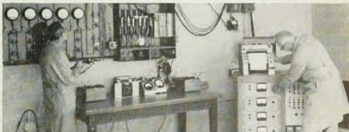
The Honeywell Model 1108 Visicorder Oscillograph in use in the Janitrol test room.
