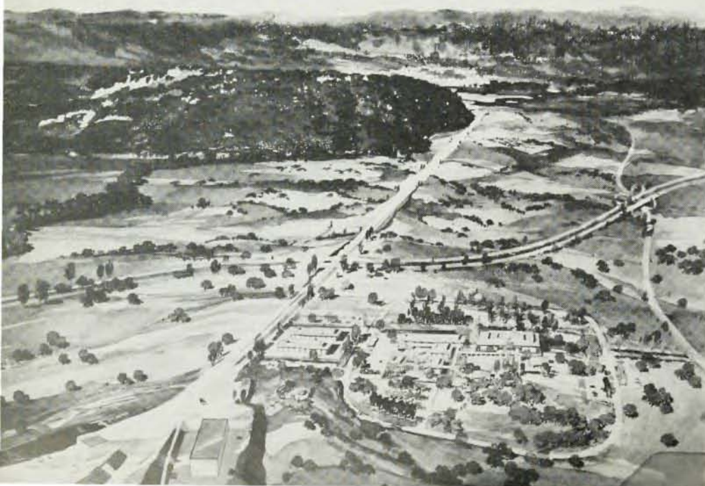
Artist's conception of the layout of the two-mile linear accelerator now under construction at Stanford university. This machine will raise electron-linac energies to the 20–40-BeV range.
