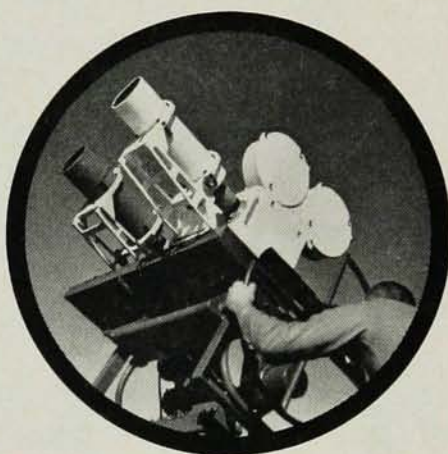
This compact 27 pound unit is a direct descendant of the versatile Model V, 70 mm MULTIDATA® camera (below).
