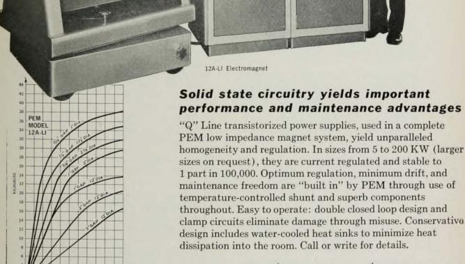
Illustrated: 12A-LI Electromagnet System. Includes magnet, "O" Line power supply, N.M.R. equipment and water-to-water heat exchanger, Pole face windings available to increase volume of uniformity
