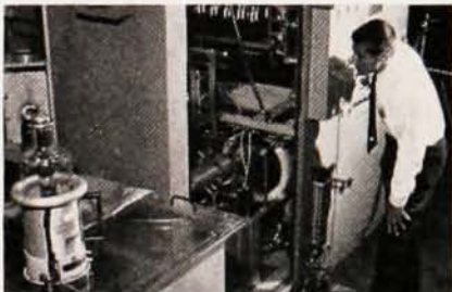
2. EQUIPMENT —A new high-power ignitron modulator—developed and built for use with Sperry Megawatt Klystrons.
