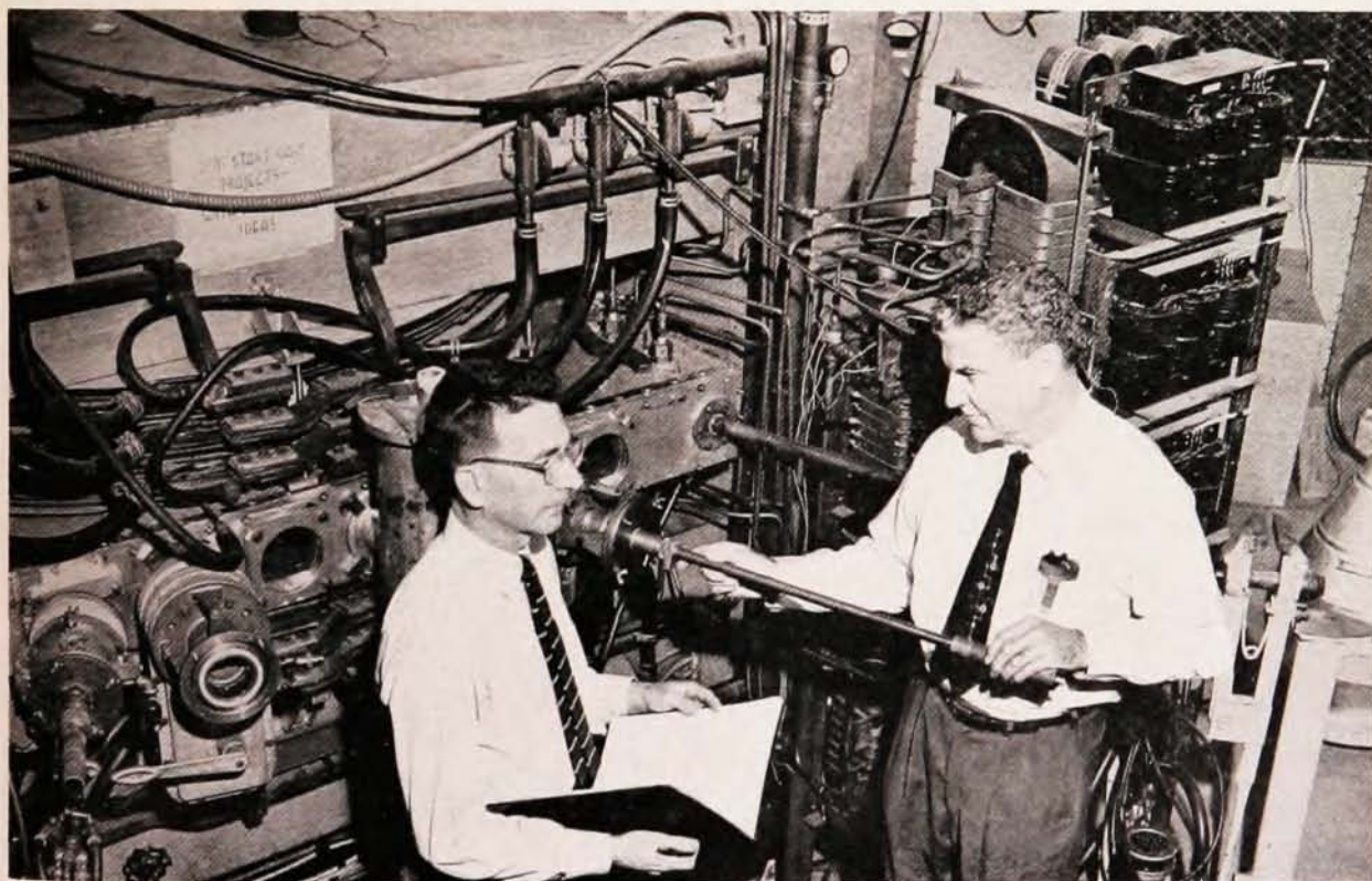
Physicists Byron T. Wright and J. R. Richardson are shown above with the constant-energy AVF cyclotron which they and their colleague Kenneth R. MacKenzie designed and constructed at the University of California at Los Angeles.
