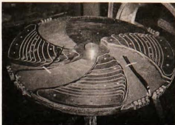
Shown above are three of the four spiral shims designed for the University of Colorado cyclotron.
