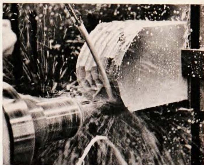
Following orders generated by an IBM computer from an AUTOPROMT program, this numerically controlled milling machine is shaping a section of a hyperbolic paraboloid.
