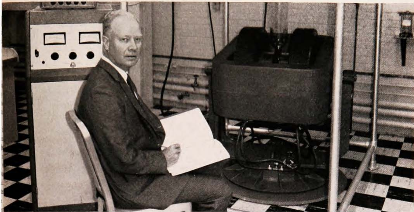
Dr. Charles F. Squire , Director of Research, with precision built 12" diameter pole face magnet being used on diamagnetic studies on alkali halides.
