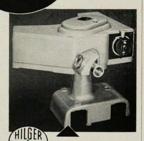
Large Aperture Monochromator for the U-V, visible, or I-R
