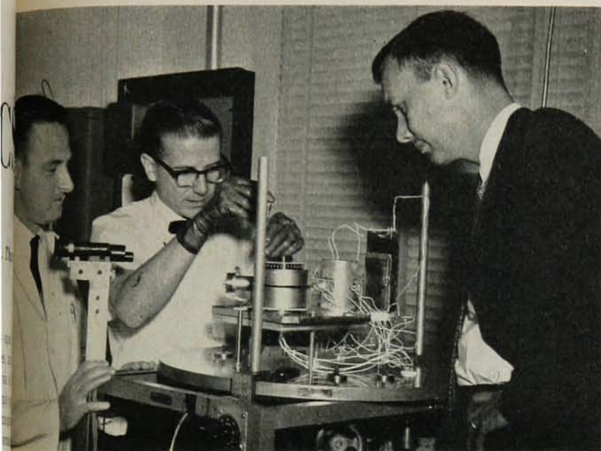
Shown (left to right) in the photograph are Lee J. Kieffer, Gordon Dunn, and L. M. Branscomb of the National Bureau of Standards group in the Joint Institute for Laboratory Astrophysics (JILA). Dr. Dunn is adjusting the scattering chamber with which he and Dr. Kieffer are studying angular distributions of protons from the dissociative ionization of molecular hydrogen. Other members of the JILA staff from the NBS Washington Laboratories are Earl C. Beaty, Peter L. Bender, George Chamberlain, Sydney Geltman, John Hall, and Stephen J. Smith. The Bureau is also represented on the JILA staff by John T. Jefferies and R. N. Thomas from the NBS Boulder Laboratories.
