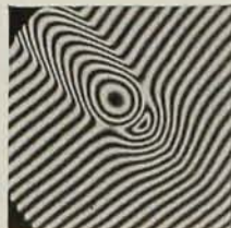
Ball track across copper crystal is narrower, harder and has higher friction in a cube diagonal direction (right interferogram) than in a cube edge direction.
