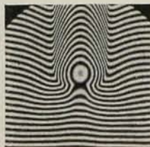
Ball track across copper crystal is narrower, harder and has higher friction in a cube diagonal direction (right interferogram) than in a cube edge direction.
