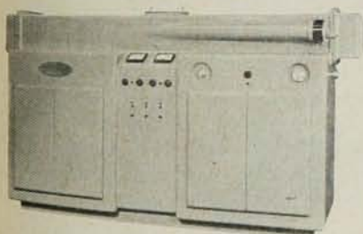
2 METER COMBINATION VACUUM U.V. SPECTROGRAPH AND SCANNING MONOCHROMATOR MODEL 240
