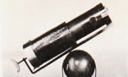
Newton's 2-inch reflecting telescope (shown in replica above) was the earliest ancestor of Mt. Palomar's 200-inch Hale telescope (below).
