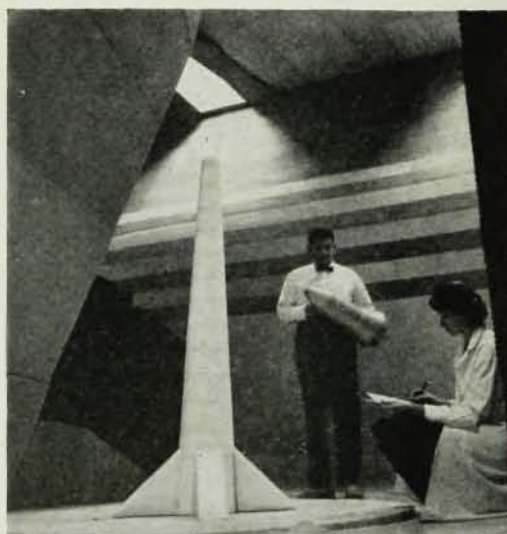
Anechoic chamber in Republic's Electronics Laboratory, equipped with remote-control turntable, is used for tests in simulated space environment.
