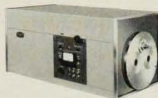
Model 78420 1 Meter Vacuum Ebert Scanning Spectrometer For direct measurement of relative line intensities in ultraviolet, visible and infrared regions. Similar to 1.83 meter Spectrometer, Model 78400, the main differences being smaller size, somewhat lower resolution and an aperture of F/8.6. Equipped with a twelve-speed scanning drive.
