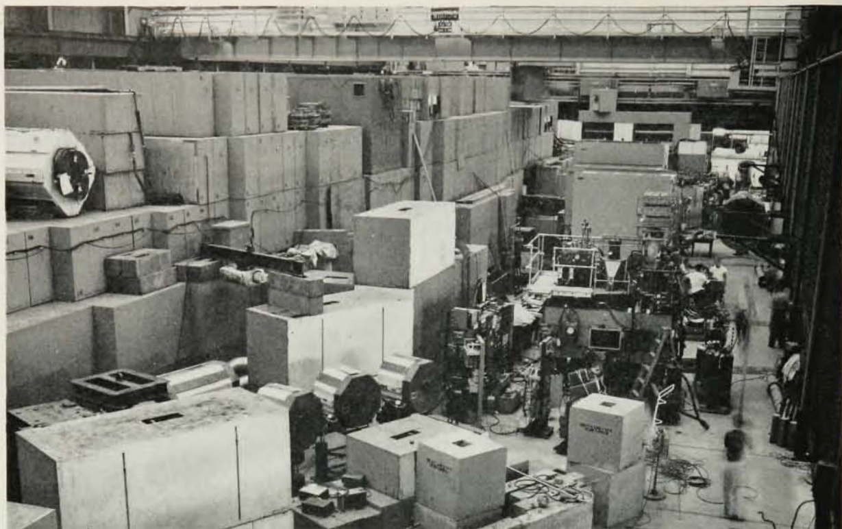
Original target area for the AGS, shown here filled with concrete shielding blocks, focusing magnets, and experimental equipment, now has ample additional space for experiments in area behind the walls to the right and in the right rear.
