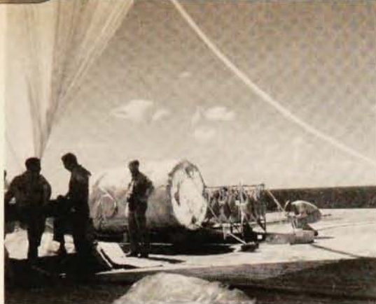
Skyhook balloon is inflated by tube while equipment is given last-minute check prior to launching. Ballast rack next to gondola carries sandbags and electronic control equipment.
