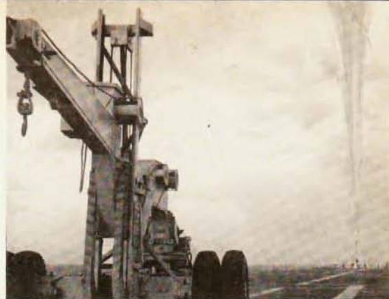
Aircraft lifting crane holds lines attached to balloon, fed through rollers on deck. During inflation crane moves forward on deck, enabling balloon bubble to expand and rise upward.
