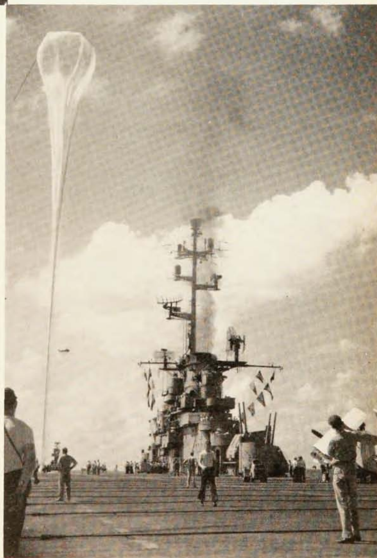
At left, with inflation tubes tied off and dangling, the Skyhook balloon "Bravo Re-Fly" is slowly fed through rollers on deck of the aircraft carrier "Valley Forge", restrained by lines running back to the mobile crane in right foreground. As seen moments before launching, below, the crane has moved forward, allowing the balloon to stand up nearly 500 feet above deck. Emulsion stack carried in the gondola had been exposed to cosmic radiation for about five hours in an earlier ascent, and during this flight received an additional 27-hour exposure at high altitude.
