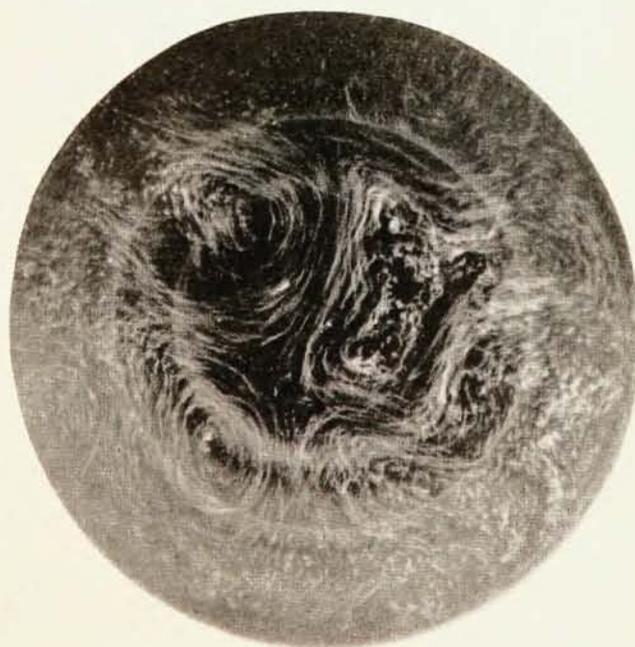
Fig. 5b. Streak photograph of surface of a mercury layer bearing a temperature gradient of about  $1^{\circ}\text{C}$  per cm, 3 cm deep, rotating at 5 rpm in an axial field of 1000 gauss. Note the large hexagonal convection cells. (*Proc. Roy. Soc.*, 1959.)
