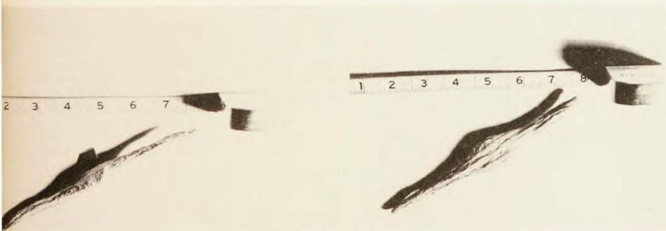
Fig. 8. A billet of solid sodium subjected to four 200- $\mu$ sec-duration "forgings" in a 100-kilogauss mirror machine. The longitudinal ridges are associated with the Kruskal-Schwarzschild instability; one can also see an oval ( $m = 2$ ) deformation. (Lawrence Radiation Laboratory, Livermore, Calif.)
