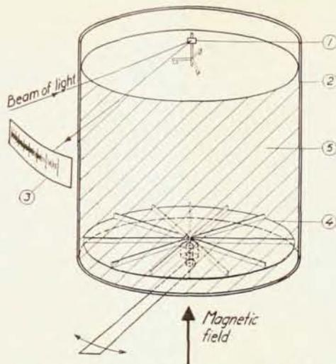
Fig. 3. Apparatus of S. Lundquist and B. Lehnert (who used two surface potential probes rather than a mirror) to demonstrate torsional cylindrical Alfvén waves. (*Phys. Rev.*, 1949.)
