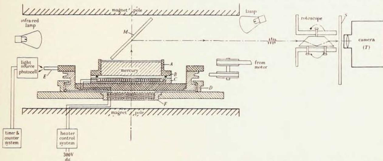
A schematic diagram of experimental arrangement. A, Bakelite cylinder; B, stainless-steel plate; C, electric heater; D, non-magnetic ball-bearing; E, stainless-steel rod; F, mercury trough; M, front-surface mirror; S, rotary shutter; T, camera.
