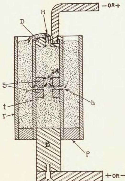
Fig. 2. Pumping liquid metals by pinch phenomenon. Cylinders  $T$  and  $t$  are insulators,  $D$  and  $B$  electrodes. Areas  $S$  are annuli to constrict the current and generate pressure. This forces the liquid through  $H$  whence it circulates through  $h$ . (*Phys. Rev.*, 1907.)
