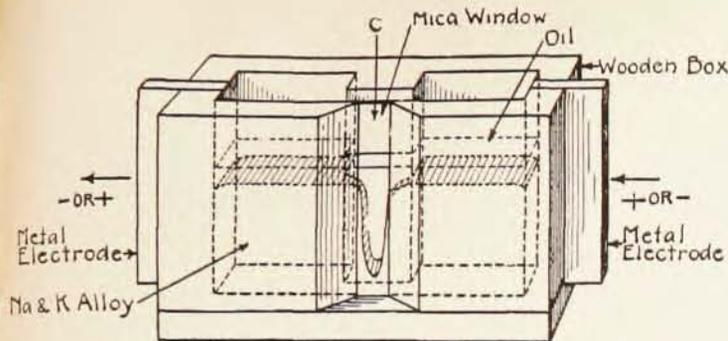
Fig. 1. Demonstration of pinch phenomenon by E. F. Northrop. (*Phys. Rev.*, 1907.)
