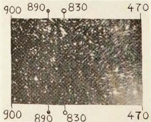
Fig. 4a (left). Apparatus used by B. Lehnert and N. C. Little to illustrate the inhibition of convective instability by a magnetic field. (*Tellus*, 1959.) Fig. 4b. Streak photograph of the motion of particles on the surface of mercury in Fig. 4a, showing regions of stability (left), instability (right), and transition (center). It was found that a normal component of 900 gauss inhibited convection at a temperature gradient of  $0.5^{\circ}\text{C}$  per cm. (*Tellus*, 1959.)
