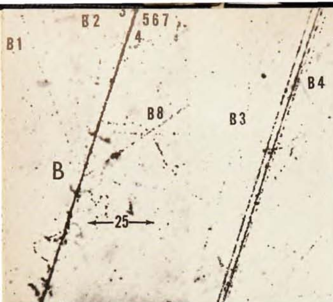
Fig. 4. Breakup of silicon nucleus into narrow-angle beam composed of a boron, a lithium, and an alpha particle (tracks 567) and four protons. Side insert shows the three heavy fragments separated a few hundred microns from point B.
