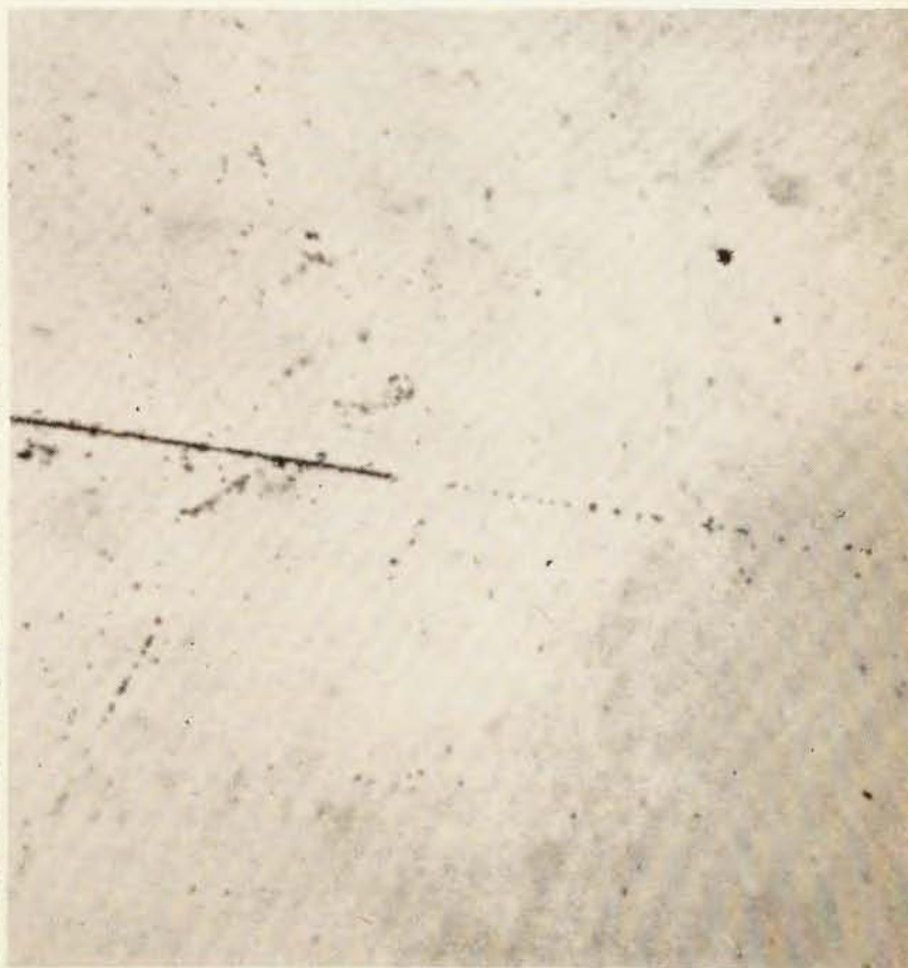
Fig. 15. Track produced by a magnesium nucleus in two adjoining layers of emulsion of different sensitivity. Portion at left is electron-sensitive G5 and exhibits the secondary delta rays. The portion at right is the Ilford G0 emulsion of identical stopping power, but devoid of sensitizer.
