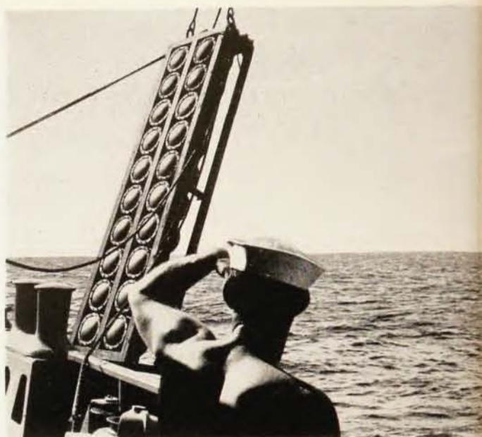
Fig. 4. An array of underwater loudspeakers provides a useful tool for exploring the use of sound waves for communication between missile launching submarines.
