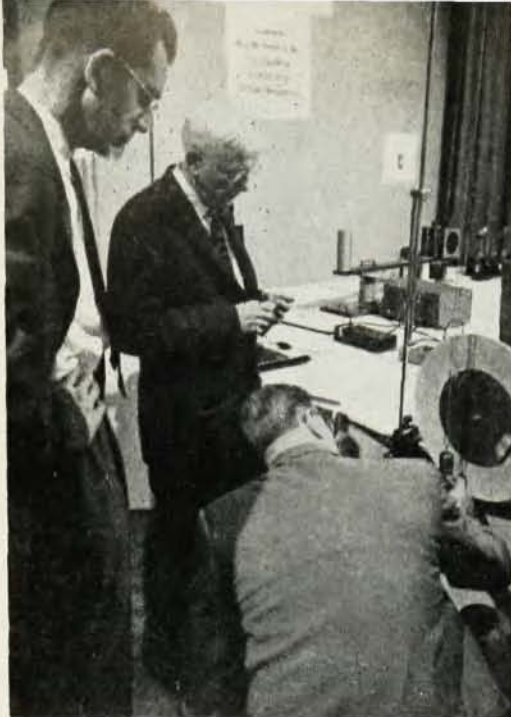
Adjustment of one of the Harvard exhibits—a circle of reference apparatus showing simple harmonic motion. In far background is device for demonstrating Doppler effect in sound; submitted by R. H. Randall of the College of the City of New York, it received honorable mention in lecture demonstration category.
