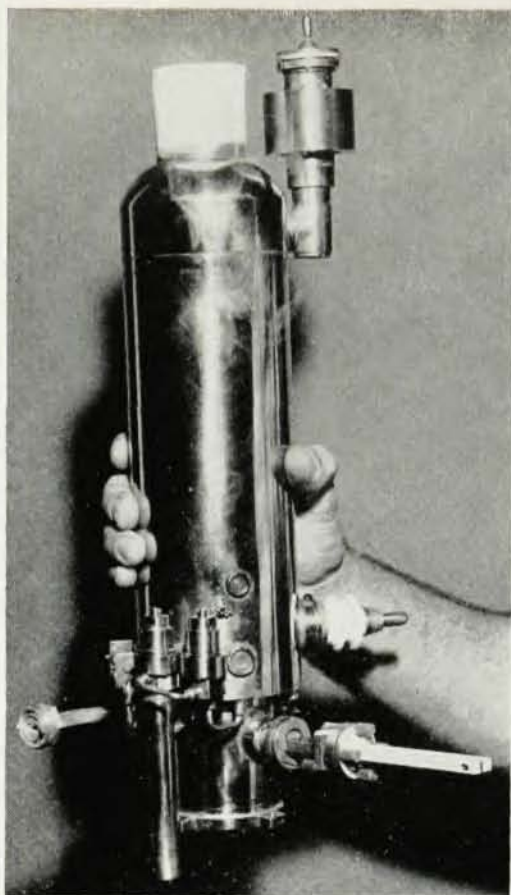
Prototype model of missile-borne maser oscillator at the Signal Corps Laboratories. Sealed off and self-contained, except for small power supply, it can provide clean k -band signal for several hours before requiring additional liquid nitrogen to maintain vacuum.
