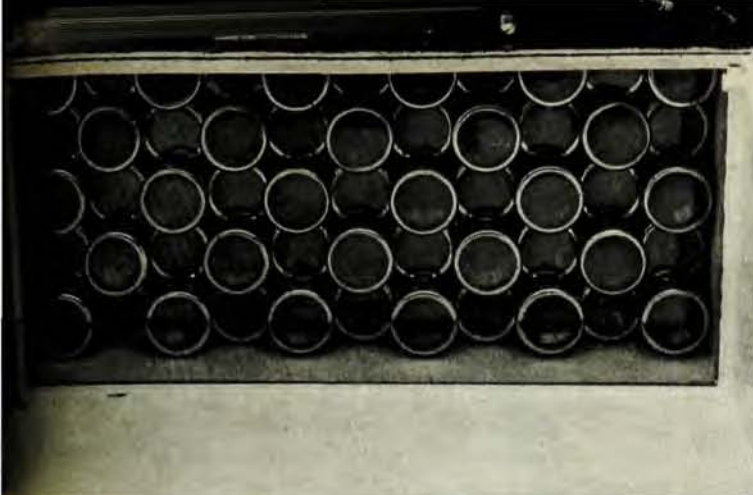
View of a tube bank of 55 photomultipliers on one end of a large detector. Tubes were staggered in order to obtain tighter packing.
