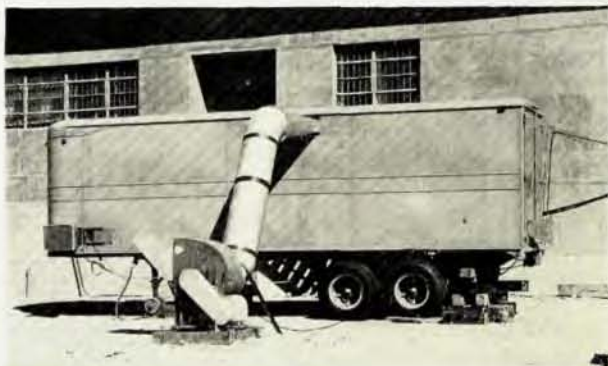
Exterior view of the electronics van showing the ventilating fan system.
