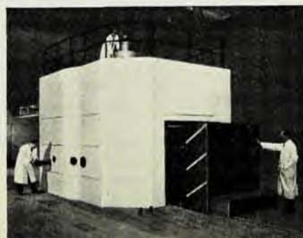
Armour Reactor is a 50 kw water-boiler unit for industrial research. It has nine beam tubes for experimental purposes.
