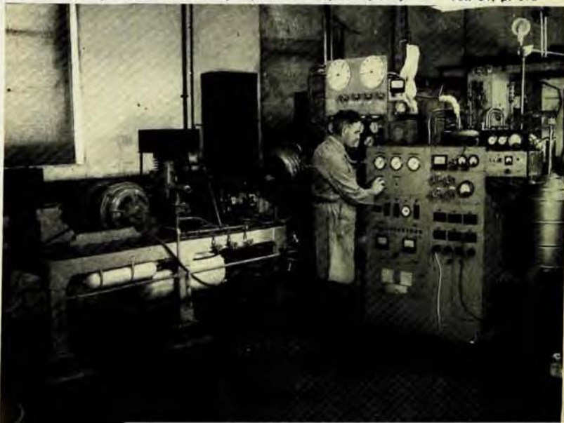
J. W. Smyth operates Collins-type helium liquifier built by Division of Physics. Because of shortage of dollars, Australian physicists frequently must build apparatus which their American colleagues usually buy. The Division has also built a mass spectrograph leak detector.
