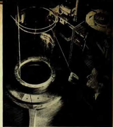
J. W. Telford operates vertical wind tunnel used for investigating coalescence between droplets in a cloud. (Division of Radiophysics)
