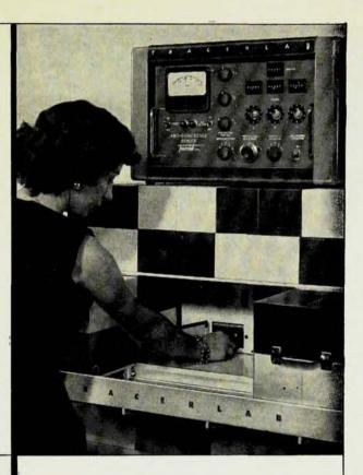
The CE-14 Low-Background Beta Counting System is complete with two central flow counters and mercury isolation shield, inside a dust-tight steel cover which also houses the anticoincidence umbrella. The massive shield, gas flow system and special three-channel anticoincidence scaler are included as an integral part of the complete system.
