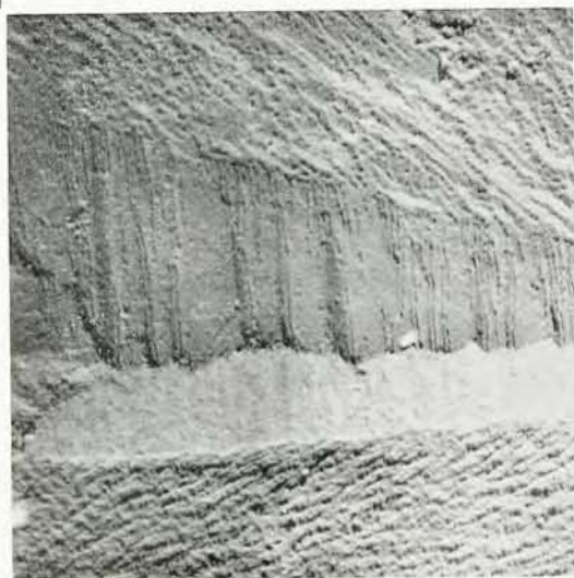
Etched Copper (16,000 \times )
