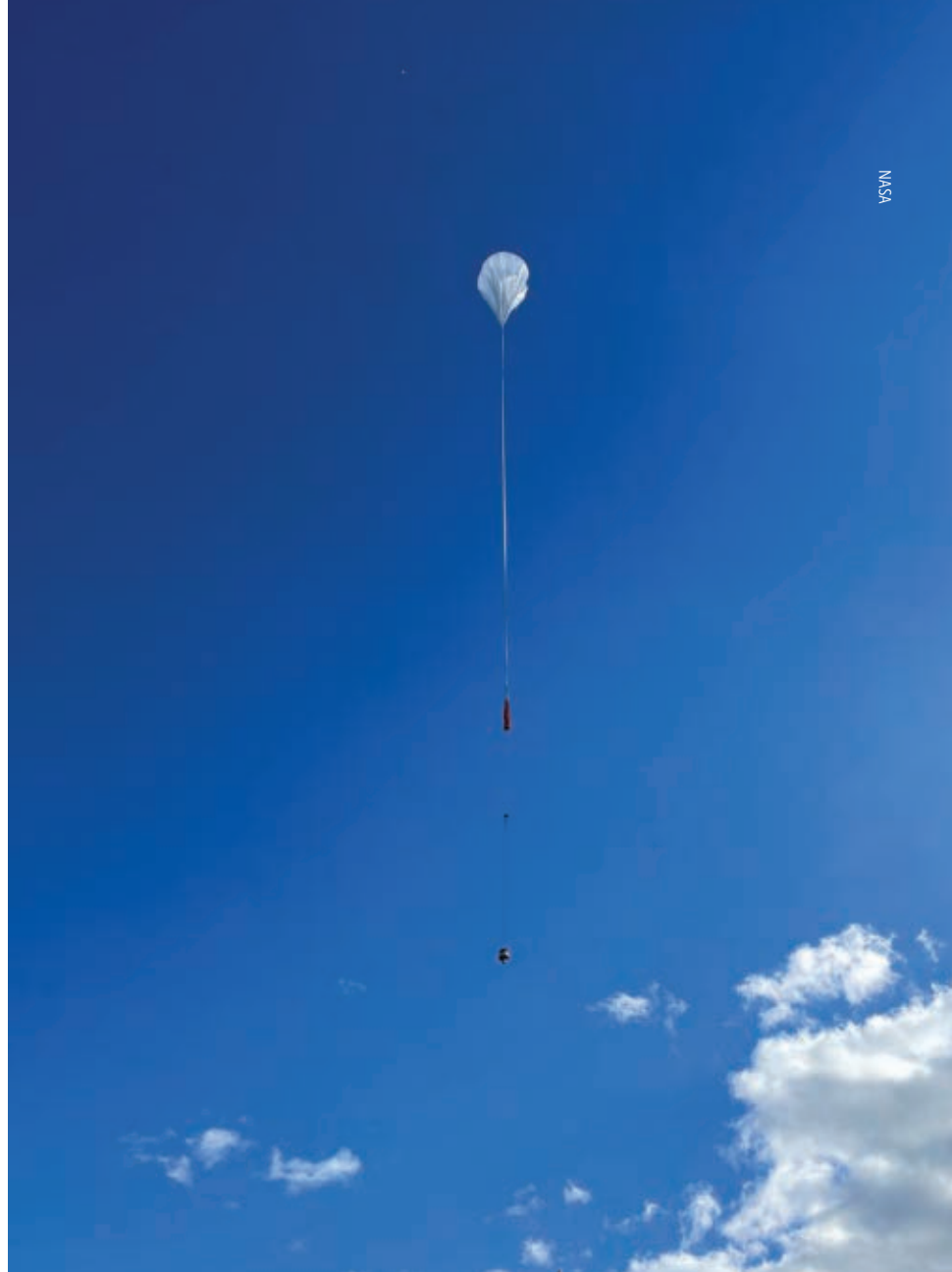
NASA'S LARGEST BALLOON , measuring 1.7 million cubic meters, ascends toward the stratosphere carrying BOOMS, the Balloon Observation of Microburst Scales experiment. It took flight on 13 July from the Esrange Space Center near Kiruna, Sweden.
