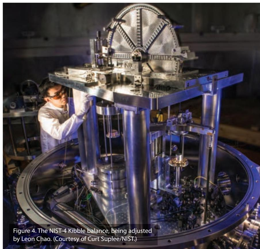
Figure 4. The NIST-4 Kibble balance, being adjusted by Leon Chao. (Courtesy of Curt Suplee/NIST.)
