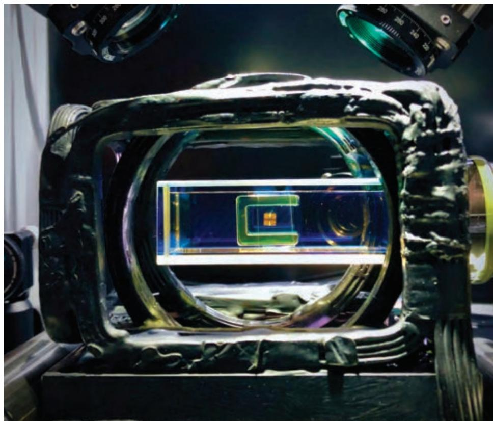
**FIGURE 1.** A VACUUM CHAMBER for trapping atoms doesn't leave much room for bulky multielement optics. By focusing light instead with a metasurface lens—the central orange square, just 4 mm on a side—researchers can make their experiments significantly more compact. (Courtesy of Ting-Wei Hsu, Scott Papp, and Cindy Regal.)
