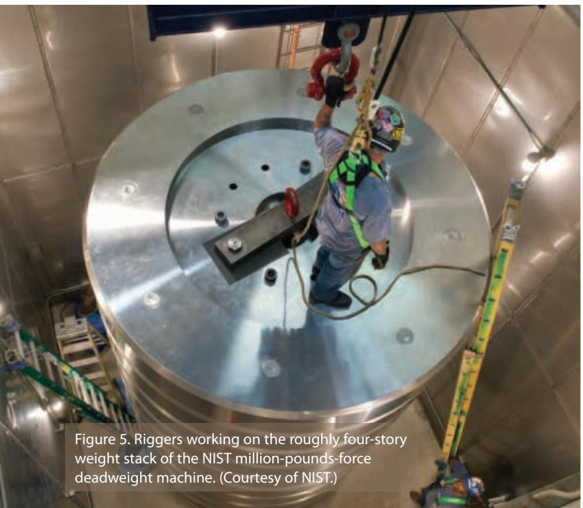
Figure 5. Riggers working on the roughly four-story weight stack of the NIST million-pounds-force deadweight machine. (Courtesy of NIST.)
