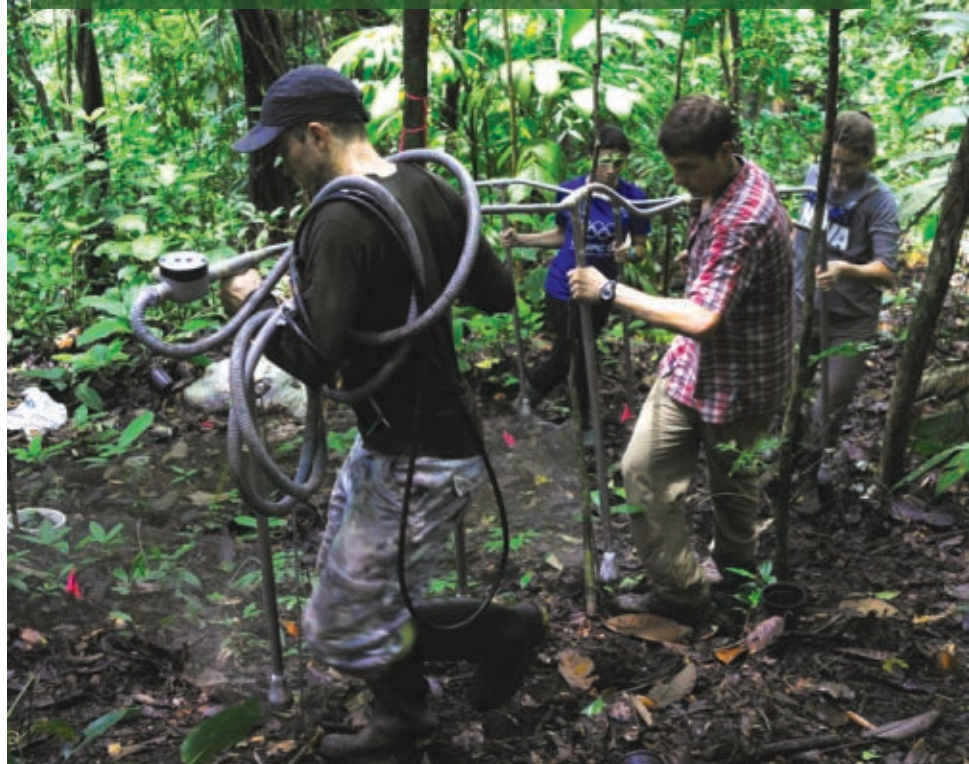
FIGURE 1. ON BARRO COLORADO ISLAND , in Gatun Lake in the middle of the Panama Canal, Andrew Nottingham and his colleagues hike through the forest with a handmade device for heating the soil. It and other instruments were buried in the ground and used to heat more than 120 cubic meters of soil by 4 °C as part of a two-year experiment to measure \text{CO}_2 released from soil in a warming climate. (Photo by Geetha Iyer.)
