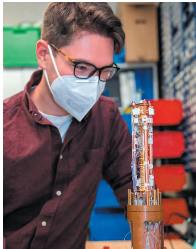
FIGURE 1. MATTHEW BOHMAN examines the core of the BASE collaboration's new cooling apparatus. The central gold-colored cylinder contains two electromagnetic Penning traps: one to hold laser-cooled beryllium atoms, the other to hold a single proton. (Photo by Stefan F. Sämmer, Johannes Gutenberg University Mainz.)
