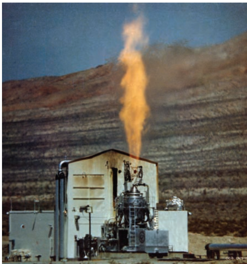
FIGURE 4. ONE EARLY TEST of a nuclear thermal propulsion reactor as part of Project Rover, which ran from the mid 1950s to the early 1970s. Here, fission-heated hydrogen propellant is exhausted into the open air of the Nevada Test Site. (Photo courtesy of the National Security Research Center at Los Alamos National Laboratory.)
